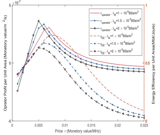
**Fig. 3.** The operator's profit and the network's energy efficiency per unit area versus the price  $\tau$  for different intensities of BSs and  $\alpha = 4$ .
