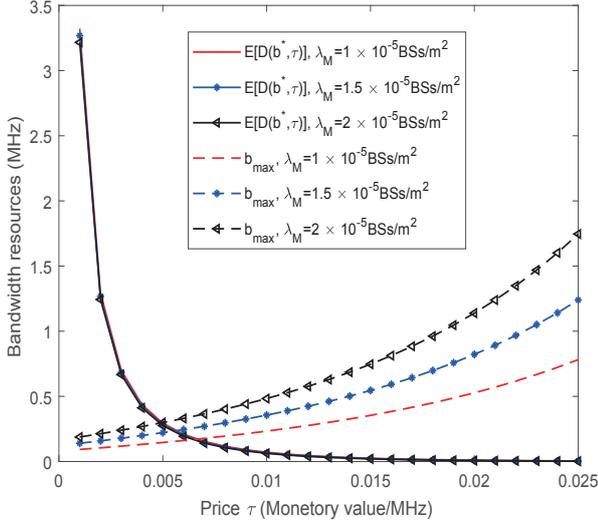
**Fig. 2.** The average actual required bandwidth and maximum allocated bandwidth per user on unit area versus the price  $\tau$  for  $\alpha = 4$ .
