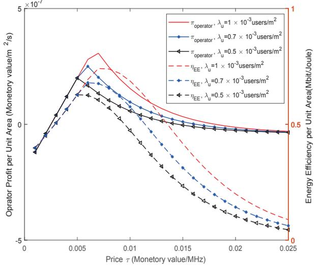
**Fig. 4.** The operator's profit and the network's energy efficiency per unit area versus the price  $\tau$  for different intensities of users and  $\alpha = 4$ .
